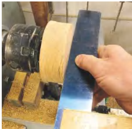
▲ Pic.5 Make sure that the base is slightly concave; this will allow it to sit on its outer edge. If you don't do this then the candlestick will be unstable
